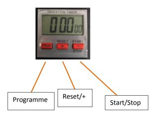
To set the timer press the 'programme' button. The seconds will flash. To adjust the time press the + and - buttons to adjust the time up or down respectively. Subsequent presses of the 'programme' button will step through from seconds to minutes to hours. Pressing the 'programme' button again will set the time. (If the digits are flashing the timer will not operate).
