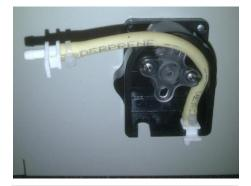
Pull the short tube out of the pump housing.
