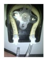
Remove the two sample tubes from the two white inline connectors
