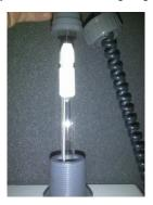
Slowly remove the lamp from the holding by lifting it vertically. Pull the lamp clear of the connector and lay it on the bench.
