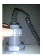
Carefully unscrew the locking ring from the top of the lamp connector.
