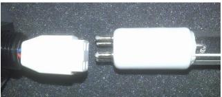
Grip the white connector and white end of the bulb between thumb and finger of each hand and carefully wiggle the two apart.
