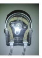
Remove the pump cover by inserting a flat screwdriver blade into one of the slots and twisting.
