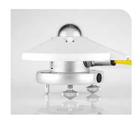
The SMP3 is a thermopile pyranometer, which differs from the technology used in the SCP which is a silicon-cell pyranometer. The difference is that silicon-cell pyranometers have high errors in cloudy conditions, whereas thermopile pyranometers have a much broader and more uniform spectral response, meaning they perform well in all weather conditions.
