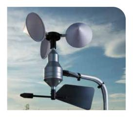
The wind speed and direction sensor consists of a low-inertia ABS cup assembly for fast response mounted on a dual ballrace-supported stainless steel shaft. The wind direction component of the sensor consists of a dynamically balanced wind vane operating a triple ballrace supported shaft and microtorque potentiometer.
