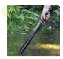
equipment at ground level. The Maji-Sonde measures the 10 standard parameters and has the ability to add up to 6 unrestricted additional electrodes.
