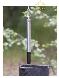
The logger collects data at user-defined intervals and stores the information in its internal memory – it can take up to 1 reading per second and store up to 500,000 readings at once. Made from titanium, the logger is built for deployment in all environments from fresh groundwater to salty marine waters. To download the recorded data, simply retrieve the logger and connect it to a PC or a handheld GPS meter.
