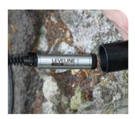
The LL-MINI is a water level and temperature sensor that provides accurate and reliable data with minimal maintenance. It is constructed using titanium and features sensitive pressure and temperature sensors. It outputs directly in SDI-12 or Modbus (RS-485) meaning you can connect it to any SDI-12 ready logging device. It has no internal power or memory, it's simply a sensor that will send data to your chosen logging device.
