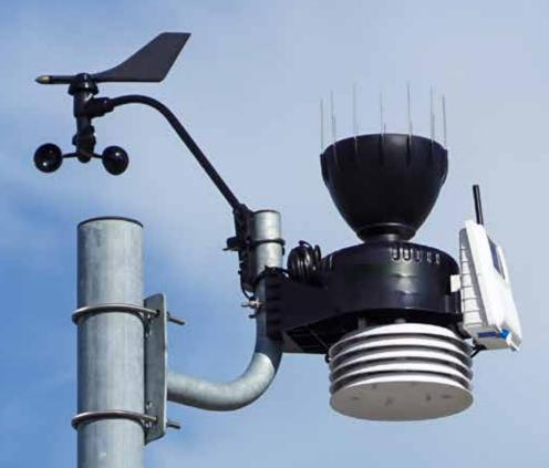
**TraceMet is a range of Automatic Weather Stations** (AWS) that have been carefully designed for the collection of accurate and reliable data on atmospheric, soil, plant and surface water conditions. With a choice of 6 models, there is a weather station for every situation. Whether you need an entry-level system for just meteorological parameters, or a premium AWS for measuring agrometeorological conditions, there is a model for you.
